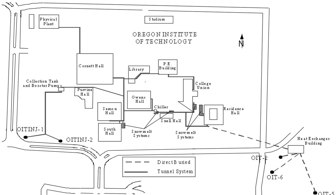
Figure 1. General layout of the OIT geothermal system.
